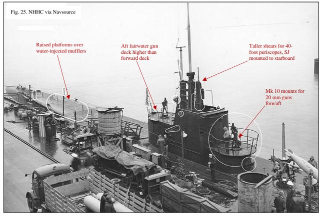
platforms indicate that these boats received new water-injected mufflers to replace the smaller units that were originally installed.
