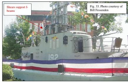
apparent, but it may have had to do with water flow vibration problems with the periscopes. Removing the covered wagon ribs during construction may have exacerbated this issue and this added bracing is how it was eventually solved for *Sailfish*. *Sculpin* was lost six months after the photo above was taken and thus never received this modification. It is likely that this is also the case with *Swordfish*, but the existing photographic record does not confirm her final configuration.
