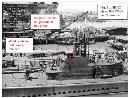
support tubes, which is now very apparent when compared to the EB versions. Note the stepped appearance of the shears due to the 34-foot #1 scope. At this point *Sculpin* retains the weld bead outlines for her hull number on the side of the fairwater. She has the Mk 5 mounts for the 20 mm
