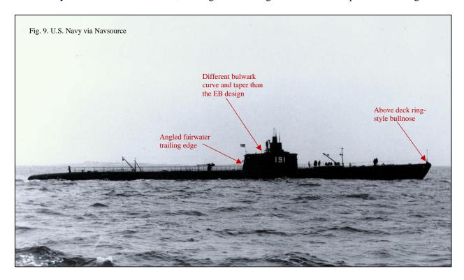
The photo above of *Sculpin* (Figure 9) shows the different shape of the upper edge of the cigarette deck bulwark, substituting the sharply curved/horizontal configuration with one that is more gradually tapered. Also, the trailing edge of the fairwater tapers at an angle to the main deck, as
