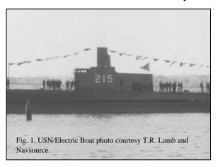
periscope shears was cut away. This was followed by the removal of the plating around the periscopes themselves. The final steps involved the cutting down of the covered navigation bridge at the forward end of the fairwater and lowering the height of the bridge itself. Not only did this
