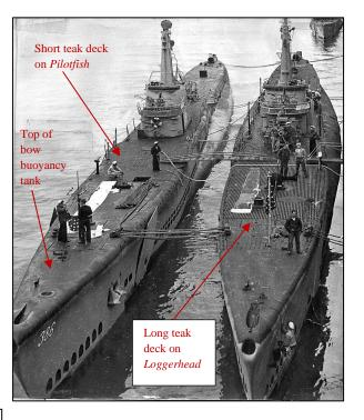
between the two designs is at the very forward end of the deck, from the jackstaff forward. The drilled steel decking stops here and is replaced by a solid surface. This area is actually the top of the bow buoyancy tank, a tank kept dry on the surface to prevent the bow from burrowing into a head-on sea. Figure 25 is a 1944 shot of *Blower*, showing the length of the EB design slat deck. It is also interesting to note the damage to her forward deck. While enroute to the Pacific in the fall
