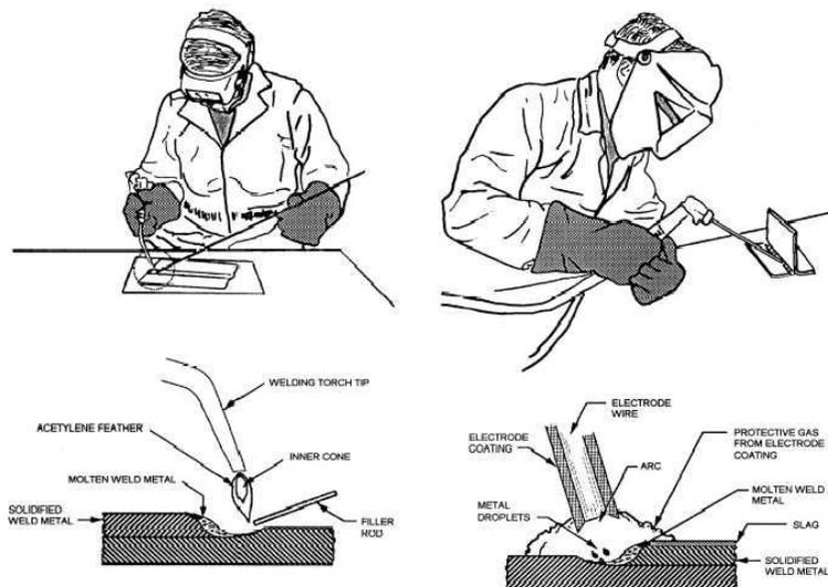
Fig. 3. Oxyacetylene and electric arc welding
