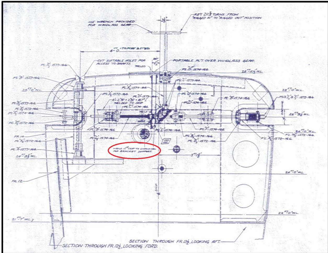
Figure 6. Construction drawing of the forward superstructure of Argonaut. Circled area contains reference to welding. (Drawing courtesy of Ric Hedman at PigBoats.com)
