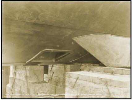
*Figure 7. View of Dolphin's keel area, showing welded flood port flange and welded bilge keel. (NARA photo courtesy Roger Torgerson and PigBoats.COM)*
