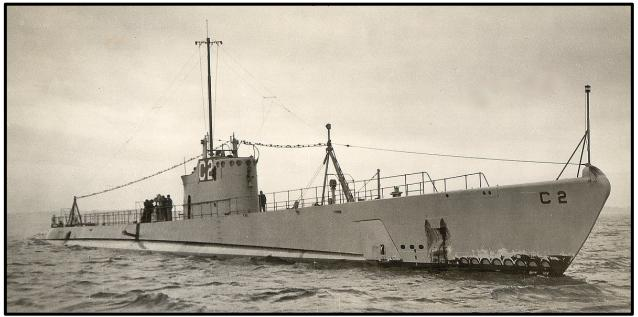
*Fig. 4. USS Cuttlefish (SS-171), 27 March 1934 on builder's trials. She is traditionally thought of as the first boat on which welding was used. (Ric Hedman via PigBoats.COM)*
